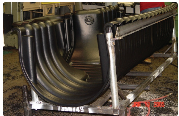
SmartDitch semi-circular tee-section channel in trim fixture.
